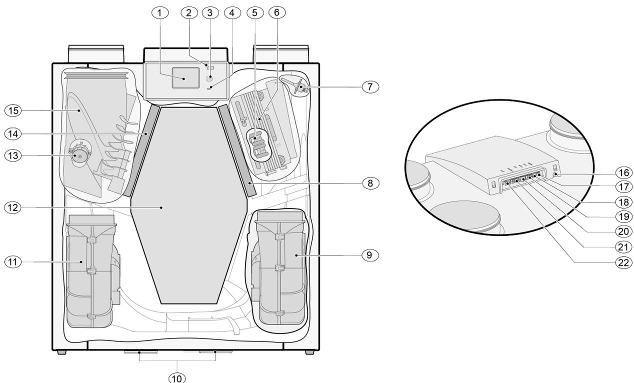
The appliance shown above is a left-hand version: in the case of a right-hand version, the connector of the preheater and the bypass valve are installed in mirror image!
