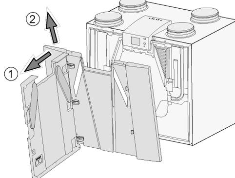
4 Remove the heat exchanger. Be careful not to damage the EPS parts in the appliance.
